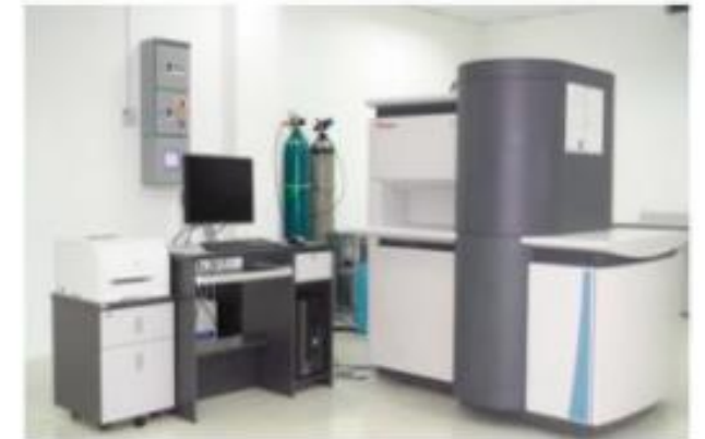
X-ray Photoelectron Spectrometer (XPS) Model: Thermo Scientific K-Alpha
